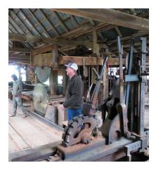
They have the box factory on a steam furnace for power, but with small orders, machinery is driven by electricity from generators or solar power. The entire property is off the grid with solar power and battery backup powering the family home.
